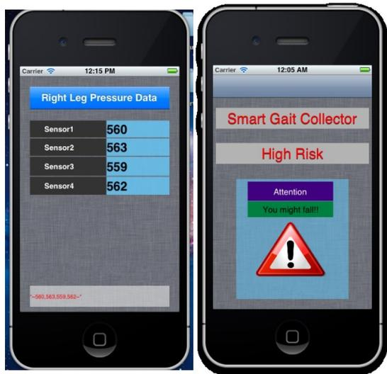
(a) Smartshoe sensors data collection interface (b) Audio alert message generation based on abnormal gait
